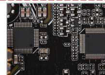
Sophisticated Multi Layer Board (Network board)
